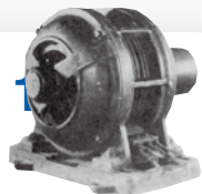
20HP three-phase induction motor (1917) Yaskawa’s first commercial product
